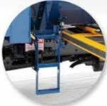
Folding ladder allows for convenient hopper access.
