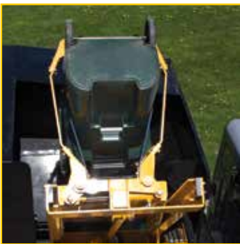
Extended debris shroud helps to keep refuse in the hopper.
