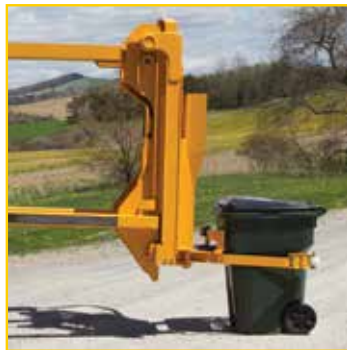
A 41" straight vertical lift before the cart tips allows for easy collection off of retaining walls and snowbanks.
