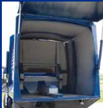
Safe horizontal ram eject unloading eliminates costly multi-stage cylinders
