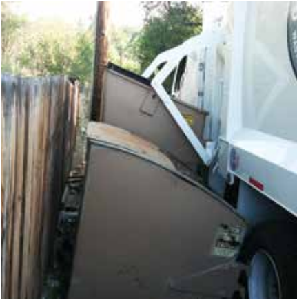
Compact lift system is designed to handle tight alley pickup
