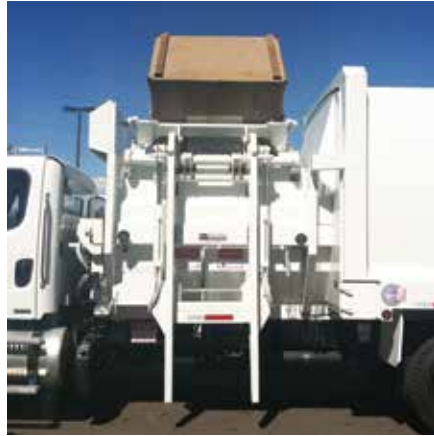
Lowest industry dump height at just 14' with a lift capacity of 4200 lbs.
